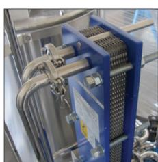
The wort must then be cooled down to fermentation temperatures before yeast is added. The wort cooling process is carried out using a plate heat exchanger.
