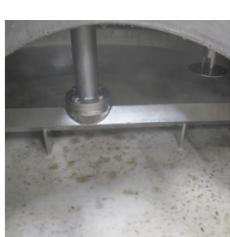
The crushed malt is added to a **mash tun (MM-LT)** and mixed with hot water to form the **mash**.
