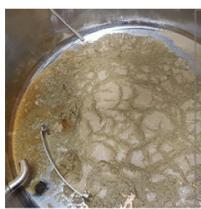
At the end of the boil, the solid particles must be separated from the liquid. When activated, the whirlpool effect makes the solid particles gather in the center of the tank bottom, so that they can be easily removed.
