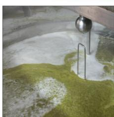
The sweet liquid called wort is pumped into the **kettle (K-W)**, where it is boiled in order to kill any microorganisms that may be present in the liquid. This is also the stage at which hops are added to the beer. Hops require boiling water in order to release their aromatic components.
